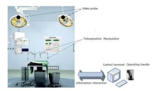
Fig. 1. The composition of the teleoperation manipulator in the spine surgery
